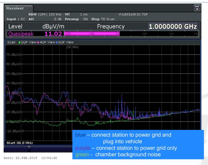
Beware of the impact of the charging station itself, shielding/filtering are needed to assure at least 6dB below limit
