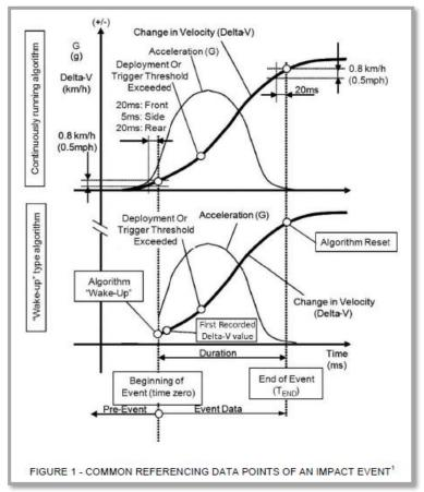
Upon detecting a specified force of impact, the airbag sensor starts recording data (but doesn't if the impact is below a specified value).
