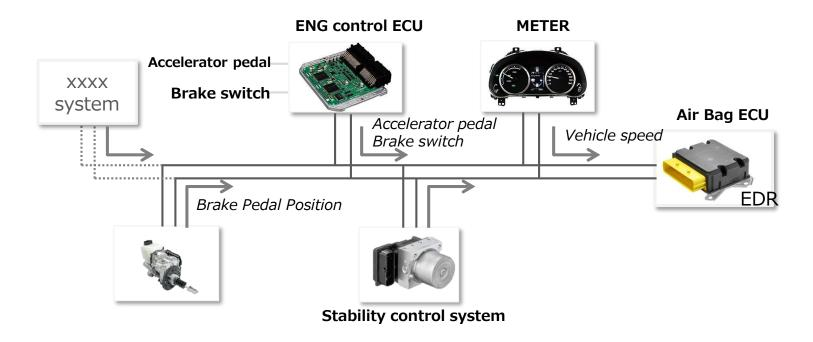
For EDR to receive and record data of other systems, the ECU of each system must be connected to CAN and data transmitted.
