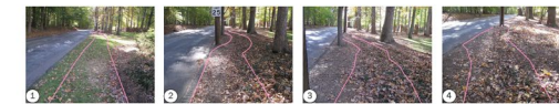
Shown above is a sequence of four pictures showing a five foot sidewalk measuring post existing trees. Porous rubber sidewalk material will help preserve trees and provide an ADA compliant surface.
