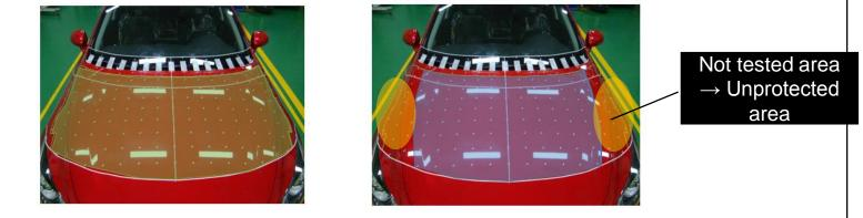
**2 Head Test Areas depending on the test method(static/dynamic) in the same car model** (Even if both are fitted with DPPS, the test area may vary depending on the result of the verification test)
