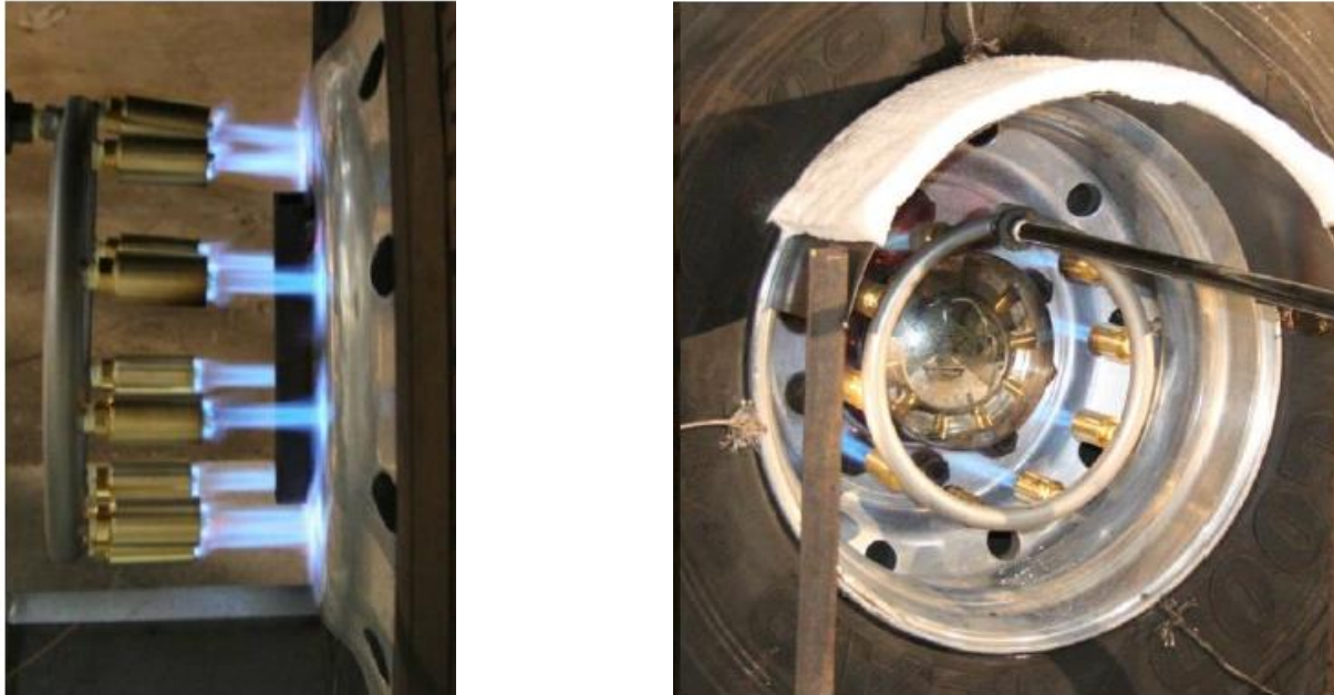
Figure 2 (Left) A photograph showing the burner pre-mixed natural gas and air torches impinging on a tag axle wheel. (Right) A photograph showing the tire shield inside a drive axle wheel rim with an insulating cover to minimize heating from the shield to the tire.
