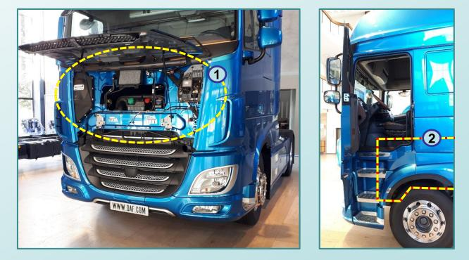
Significant lower vision lines conflict with installation of required components (e.g. cooling system) (1, engine space (2), etc.
