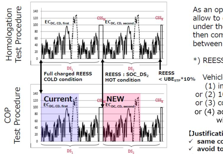
conduct one applicable cycle with fully charged battery, then compare with EC<sub>DC, CD, first</sub> between Homolo. and COP
