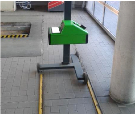
Figure 36: HBS with guide rails which are not being used
