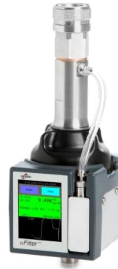
Dekati® eFilter™ operating principle is a combination of two separate measurements; gravimetric filter holder (on the left) and real-time measurement with diffusion charger and electrometer (on the right).
