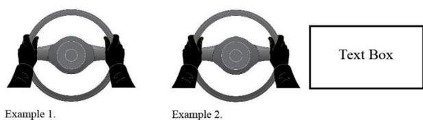
6.4.3.2. With the start of the minimum risk manoeuvre, the given signal shall change its characteristics to emphasize the urgency of an action by the driver. e.g. by red flashing of the steering control and moving hands of the pictorial information.
