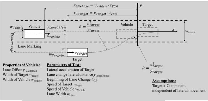
Tests shall be performed according to the parameters as shown in the table below. Each test is passed when the requirements of paragraph 2.5.4.2. and 2.5.5.2. (avoidance as function of  $t_{tC,intrusion}$ ) are fulfilled.
