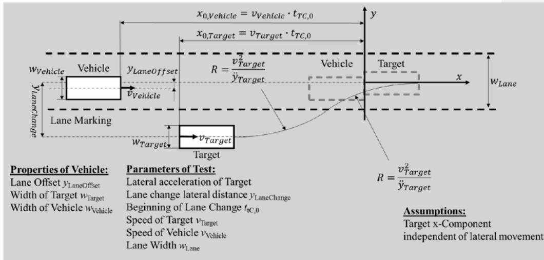
Tests shall be performed according to the parameters as shown in the table below. Each test is passed when the requirements of paragraph 5.2.4.2.2-5.4.2 and 5.2.5.2.2-5.5.2: (avoidance as function of  $t_{C,intrusion}$ ) are fulfilled.
