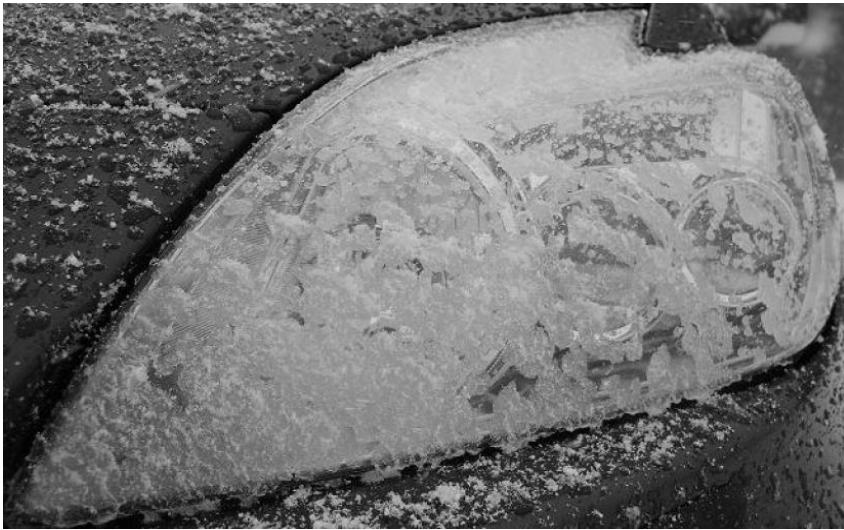
(a) soiled by snow stuck accretion
