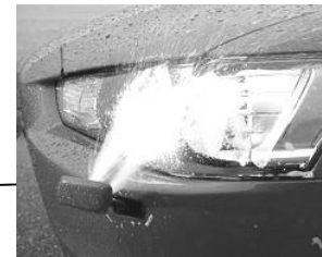
Fig.1 Appearance of headlamp cleaner system
