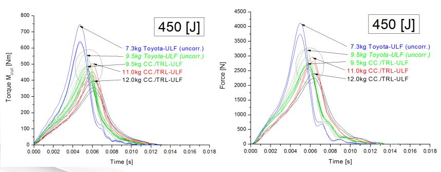
**Rem.:** At energies >=400 Joule, the continuous increase of the signals, towards higher impact-velocities, or lower ULF-masses, seems to be interrupted (see dashed circles)!
