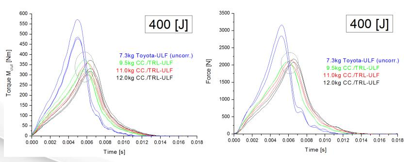
**Rem.:** At 400 Joule, the continuous increase of the signals, towards higher impact-velocities, or lower ULF-masses, seems to be interrupted (see dashed circles)!
