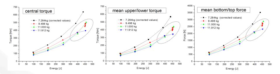
**Rem.:** At energies >=400 Joule, the continuous increase of the signals, towards higher impact-velocities, or lower ULF-masses, seems to be interrupted (see dashed circles)!
