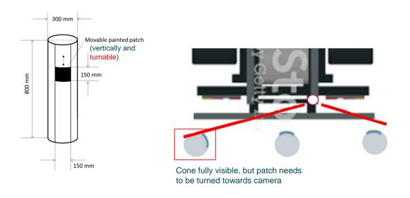
A 0.15 m x 0.15 m area or the top of the test object shall be visible at least at one position on each test object
