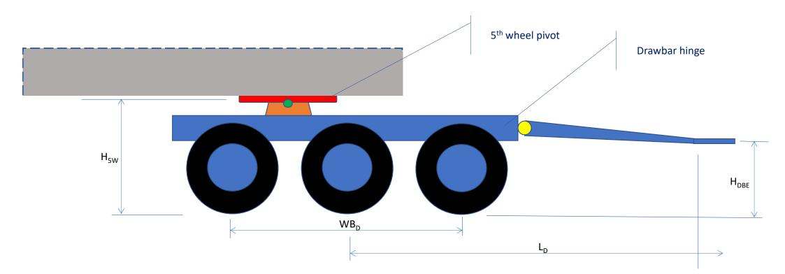
This dolly is with some pitching constraint due to long wheelbase,  $WB_D$ . Moving the 5<sup>th</sup> some distance aft could balance a braking pitching moment.
