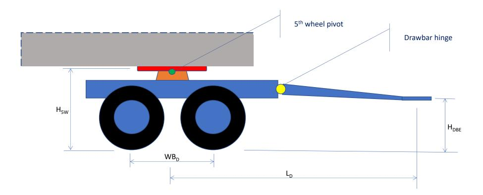
This dolly is with limited pitching constraint thanks to 5<sup>th</sup> wheel pivot axle, drawbar hinge and a short wheelbase, WB<sub>D</sub>.
