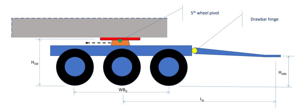
This dolly is with some pitching constraint due to long wheelbase,  $WB_D$ . Moving the 5<sup>th</sup> some distance aft could balance a braking pitching moment.
