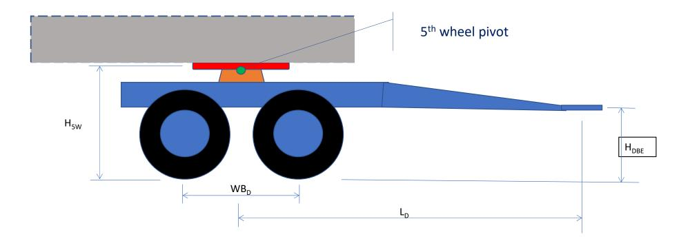
This dolly is partially pitching constrained through the rigid drawbar
