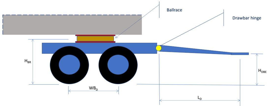
This forward axle group is fully pitching constrained to the trailer frame through the ball race
