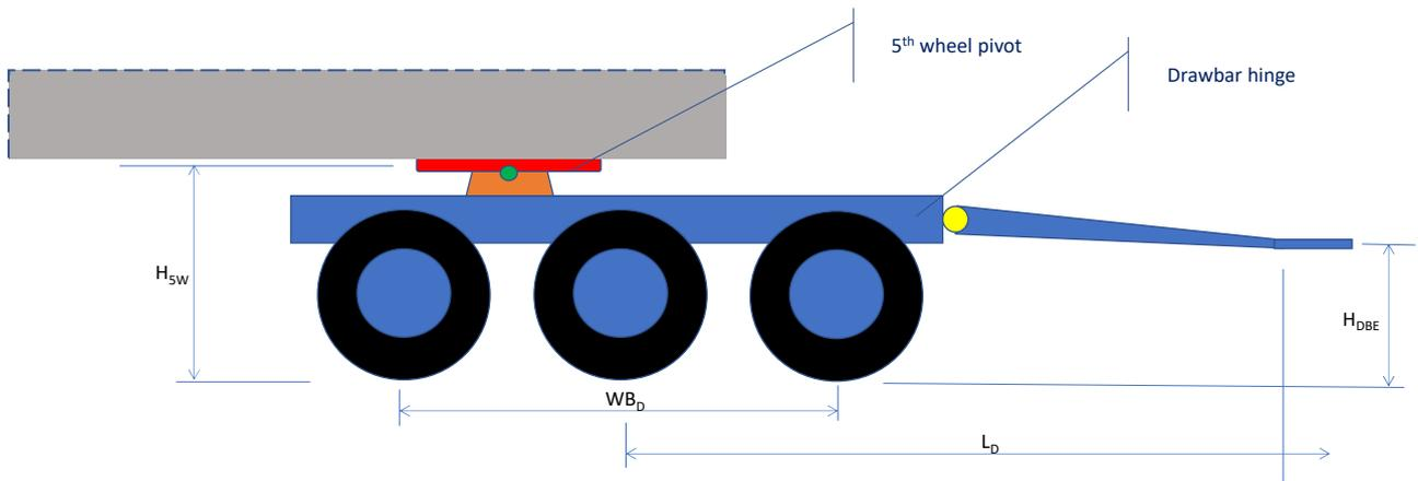
This dolly is with some pitching constraint due to long wheelbase,  $WB_D$ .
