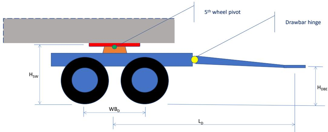
This dolly is with limited pitching constraint thanks to 5<sup>th</sup> wheel pivot axle, drawbar hinge and a short wheelbase,  $WB_D$ .
