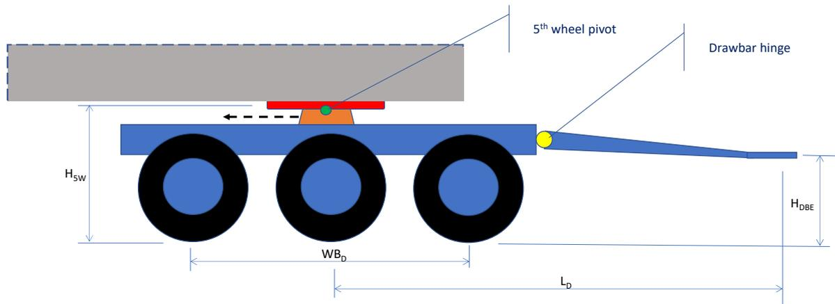
This dolly is with some pitching constraint due to long wheelbase,  $WB_D$ .
