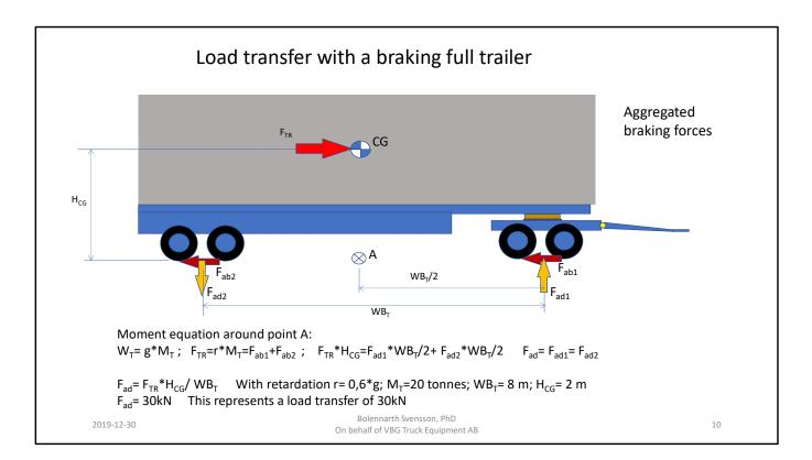
This slide just reflects the load transfer forces in a braking.
