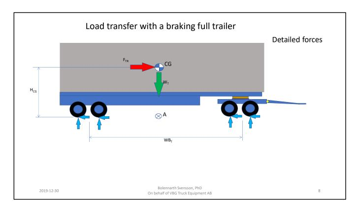
An overall detailing of the forces of a full trailer.
