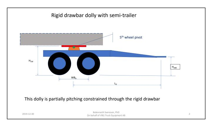
A 5th wheel has a pivoting axle. This enables the forward axle group i.e. the dolly, to pitch with respect to the trailer frame. However the rigid drawbar is supported in the clevis coupling of the towing vehicle. Thus the pitching mowement of the dolly is to some extent constrained.
