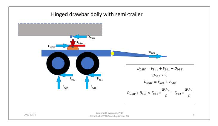
Considering the hinged drawbar the moment equation from the previous page shows the load transfer between dolly axles.
