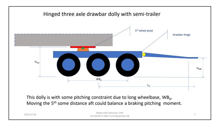
An off center position also reduces the load carrying capacity benefit.
