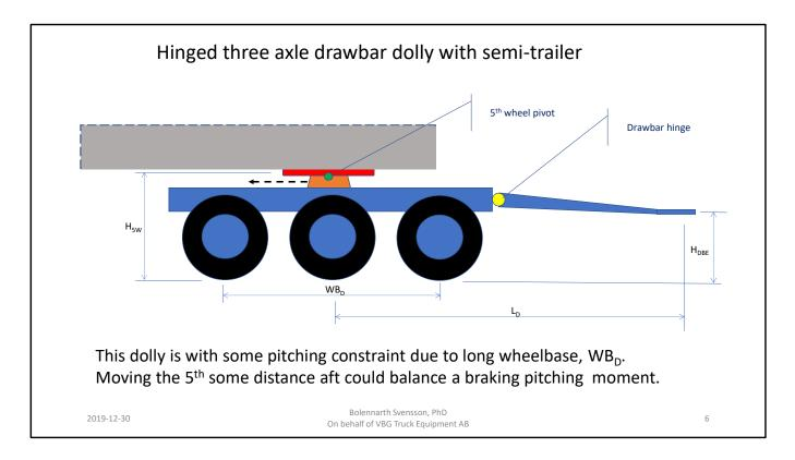
Apart from allowing more vertical load (U) from the semitrailer a three axle semitrailer results in a wheelbase that is two times so long as compared with a twoaxle dolly. An unsymmetric position of the 5th wheel gives aneven load distribution of the axles loads for the dolly. In addition it can give a counter balance to the pitching moment from braking.
