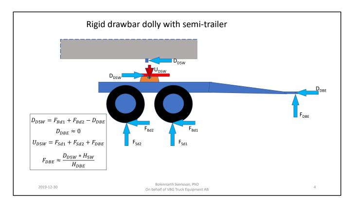
Splitting up the geometry the acting forces can be visualized. Through a moment equation around an axle in the ground surface right between the dolly axles the vertical support force of the drawbar eye can be calculated. It is assumed that the trailer is braking itself i.e. D<sub>DBE</sub> becomes zero.
