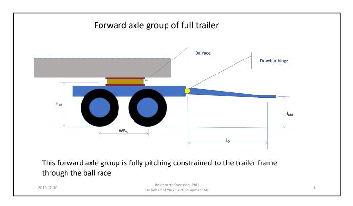
A full trailer has a ball race that attaches the forward axle group to the trailer frame. This constrains the forward axle group from pitching without bending the trailer frame.
