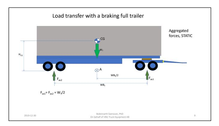
This is just an illustration of the static load distribution.
