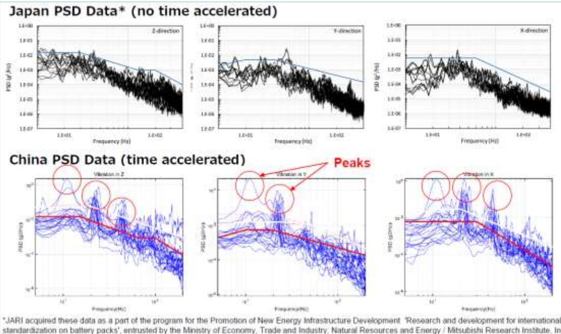
Resonance peaks at different frequencies in different directions can be seen, suggesting vibration test in 3 directions makes sense
