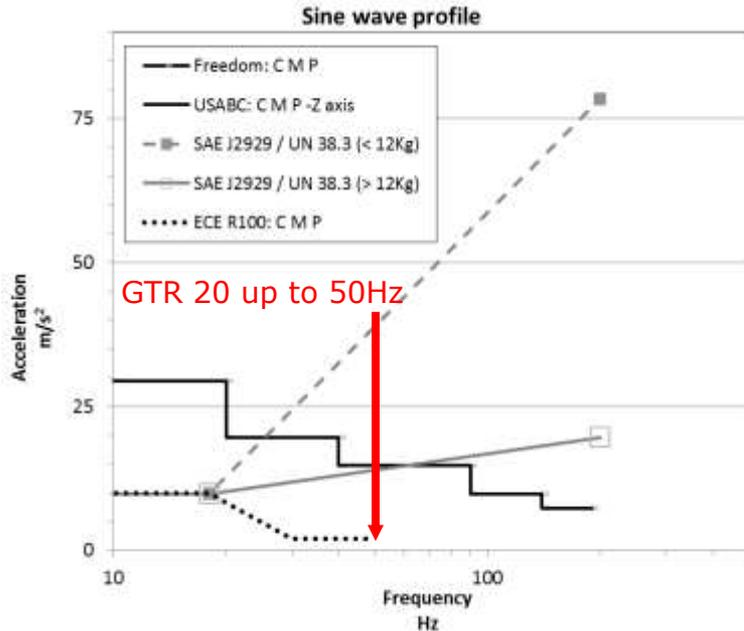
Comparison of sine wave testing profiles for various standards and regulations (Adapted from Ruiz et al. (2018))
