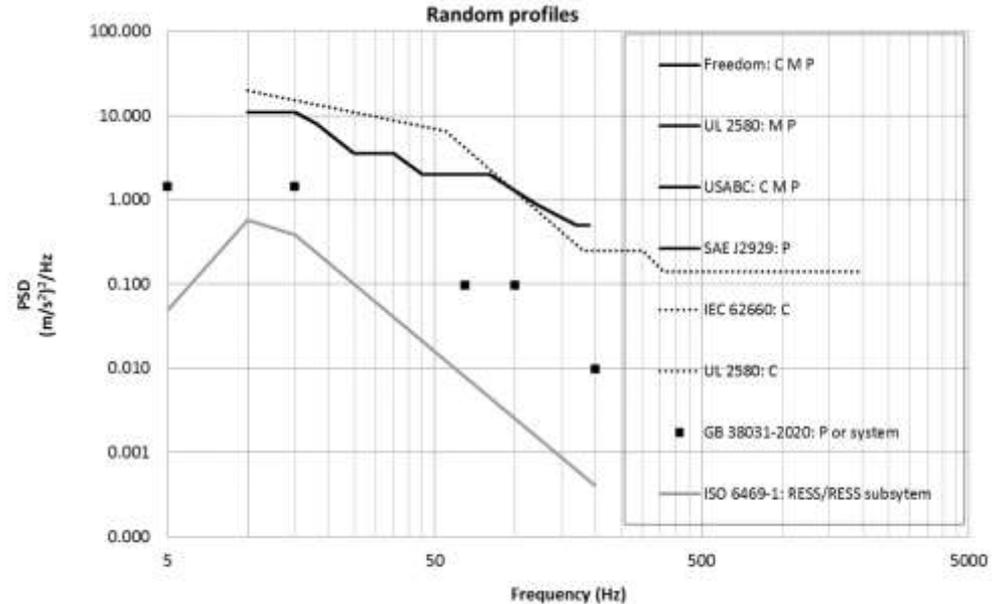
Comparison of random vibration profiles (PSD vs. Frequency – logarithmic plot) for various standards and regulations
