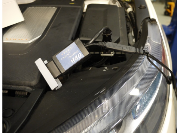
Figure 76: Wireless diagnostic adapter integration with developed battery diagnostic port
