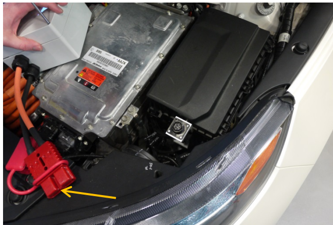
Figure 59: Developed prototype connector for high-voltage terminal access
