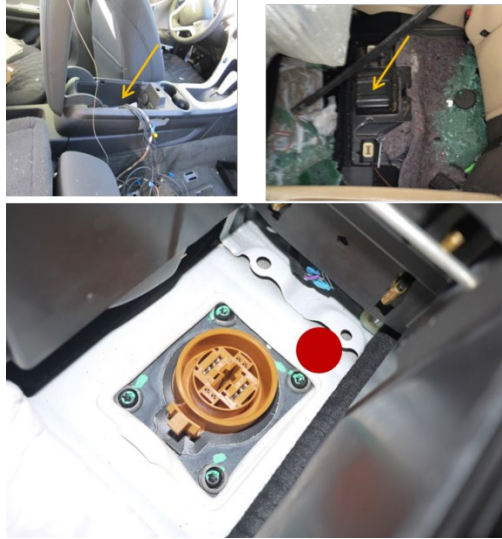
Figure 57: Diagnostic Port Location Suggestions Top left: within center console, top right: under rear seat (with metal cover), bottom: colocation with MSD
