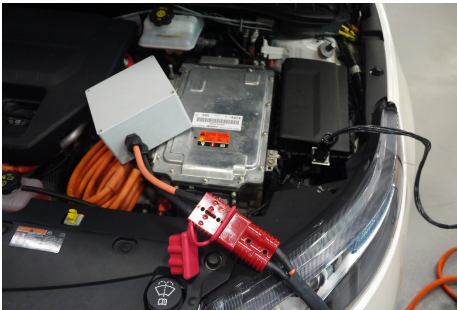
Figure 71: High-voltage and diagnostic interface port connections
