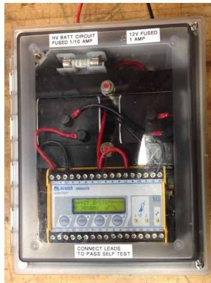
Figure 78: Offline isolation monitoring prototype tool
