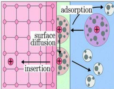
Intercalation process at the cathode-electrolyte interface
