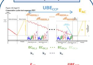
$$EC_{WLTC} = \frac{E_{AC}}{PER_{WLTC}} \qquad PER_{WLTC} = \frac{UBE_{CCP}}{EC_{DC,CCP}}$$
