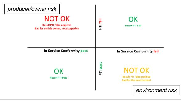
Pass/fail criteria of the PTI test must be related to the pass/fail criteria of the in-service conformity or type-approval test but less stringent.
