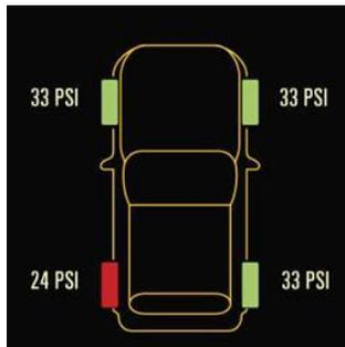
The TPMS system will warn the user in case it detects a drop in inflation pressure below the system-defined threshold limits.
