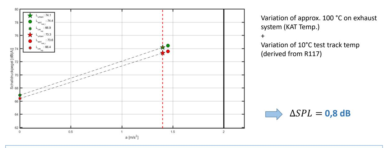
High-performance vehicles in particular can have a large dependency on component temperatures of the power train. Here, too, the source distribution decides how large the influence on the end result is.
