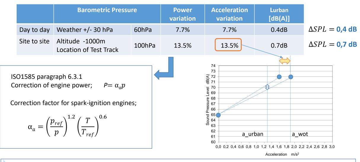
The influence of barometric pressure can be calculated by using ISO 1585 "Engine test code – Net Power" (or R85)
