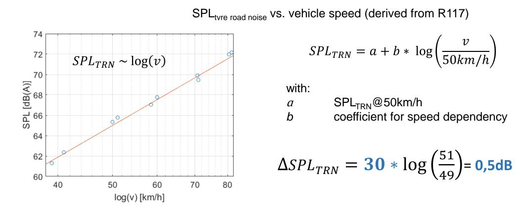
Assumption for calculation: mean coefficient of the speed dependency is 30 (usually varies between 27 -33 for C1 tyres). Depending on the source distribution this effect influences the test result of crs and wot measurement.
