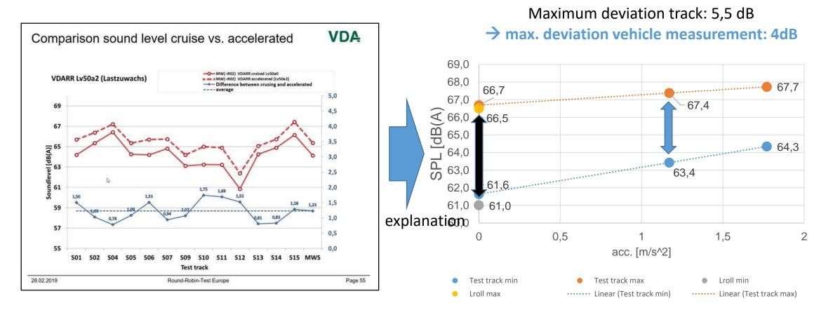
Different test tracks surfaces lead to different tyre road noises. Depending on the source distribution they influence the test result of crs and wot measurement differently.
