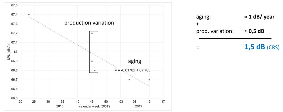
The variation of 0,75 dB in WOT measurement assumes a source distribution between tyre road and power train noise.
