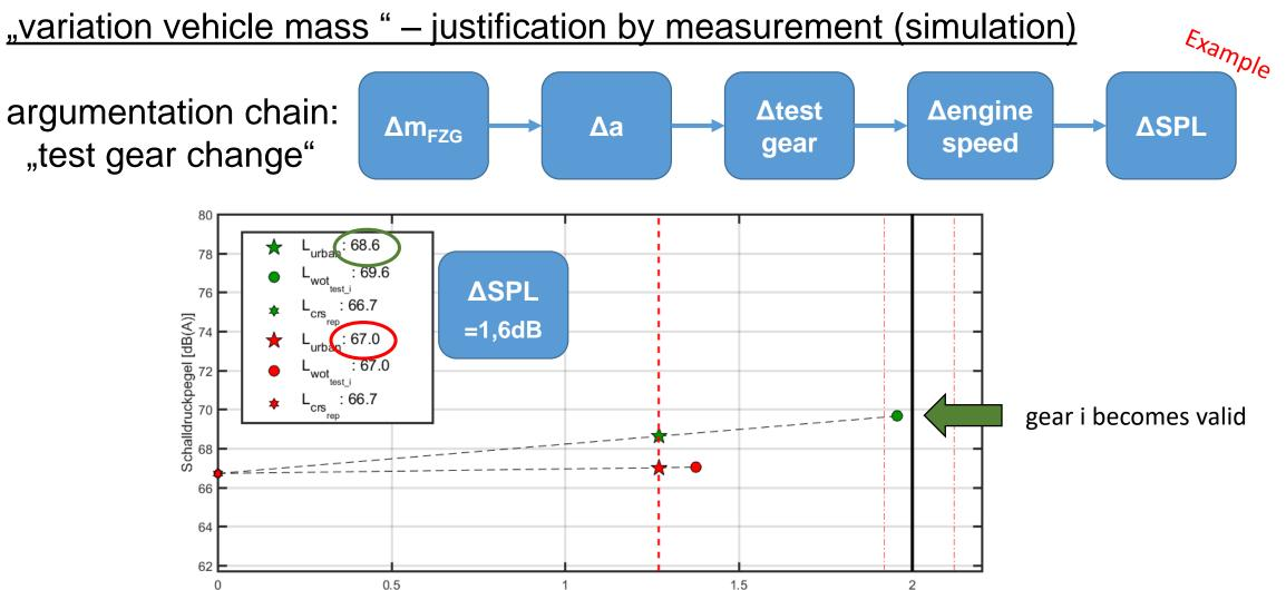
The main impact of the variation of the vehicle mass is on acceleration behavior and can cause a test gear change. The test gear change leads to another test engine speed and another sound emission.
