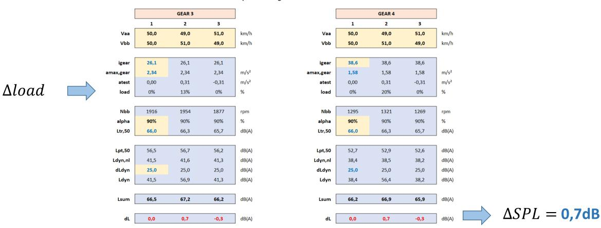
Influence of vehicle speed and engine load variation on cruise test result
