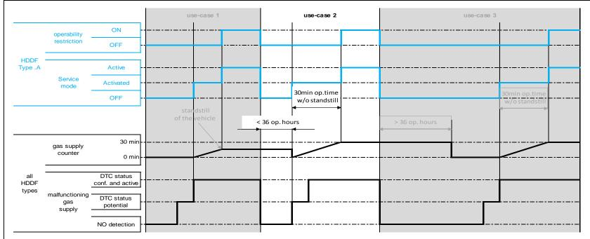
A malfunction of the gas supply is detected while the gas supply malfunction counter is not at zero (in this use-case it indicates the value it reached in use-case 1 when the vehicle became standstill).
