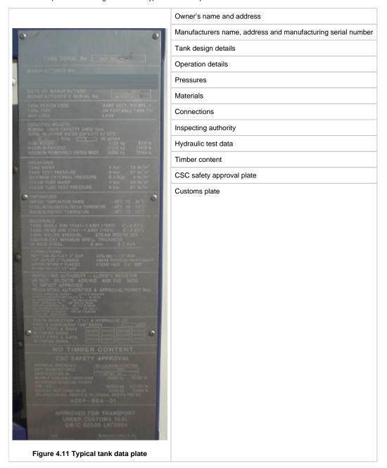
The important sections are the CSC safety approval plate and the hydraulic test data. Every tank should be subjected to a pressure test every 30 months and a full hydraulic test every 5 years and the date of the test marked on the data plate.
